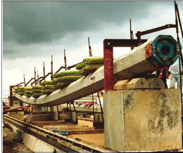
Fig. 7.43 Verifying the principle of the curvature probe
