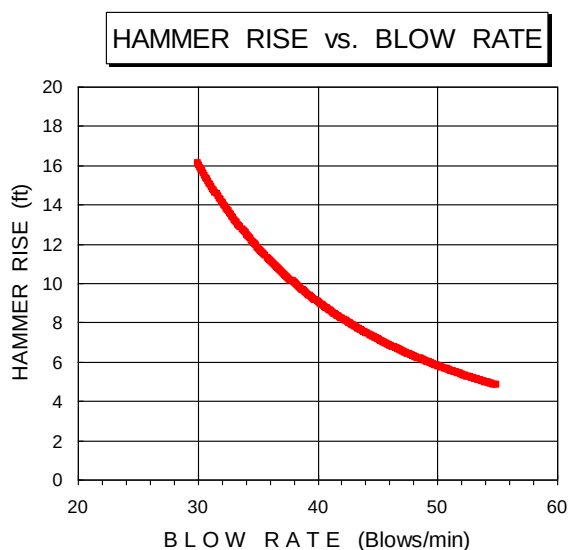
Fig. 9.7 Hammer rise (ft) as a function of blow-rate (BPM). Single-acting diesel hammer. Effect of friction in ram cylinder is not included)
