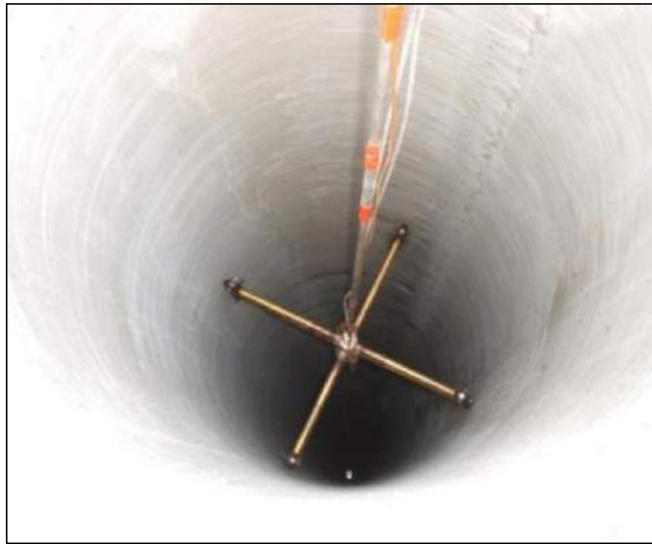
Fig. 8.24 A Glostrex gage placed down in a cylinder pile (Hanifah and Lee 2006)
